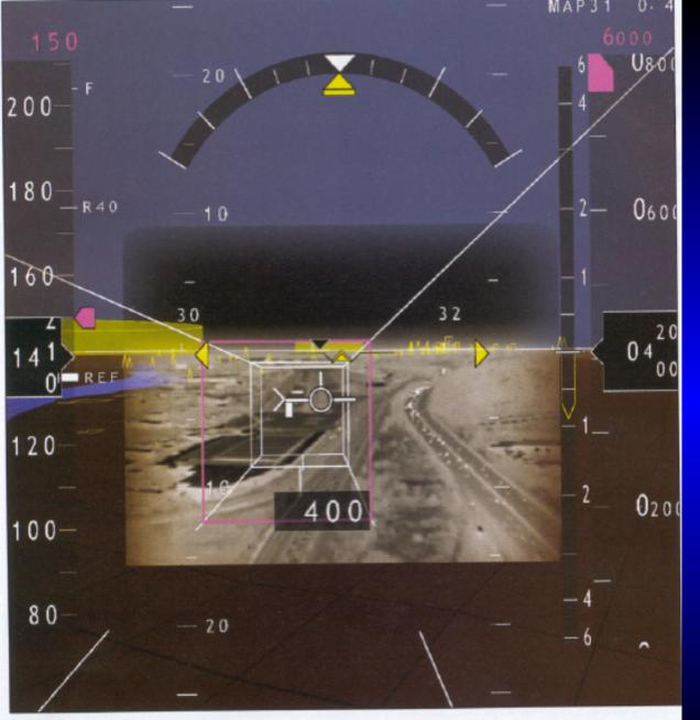
Fusion of the SVS PFD with infrared enhanced vision is another innovation from the Rockwell Collins team. In this view, the pilot can see his 3D pathway in the sky, obstacles in the SVS database and IR EVS imagery—the actual terrain in front of the aircraft—in real time. Rockwell Collins
