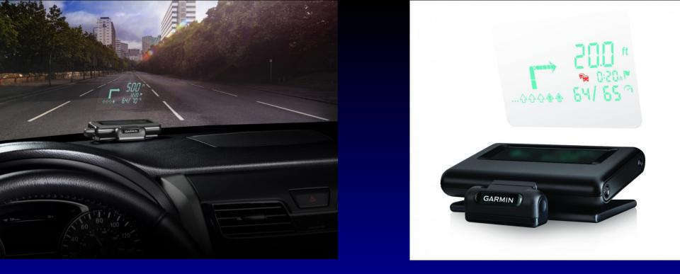
Garmin's pocket-sized, portable HUD wirelessly connects to a smartphone running a navigation app, and throws directions and useful information onto the inside of the windshield
